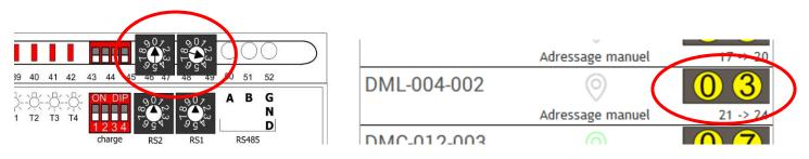
▲ The DMC-008-001 modules with a lower software version than V1.25 must be manually addressed via the coding wheels. (you find the version in menu 7.10)
