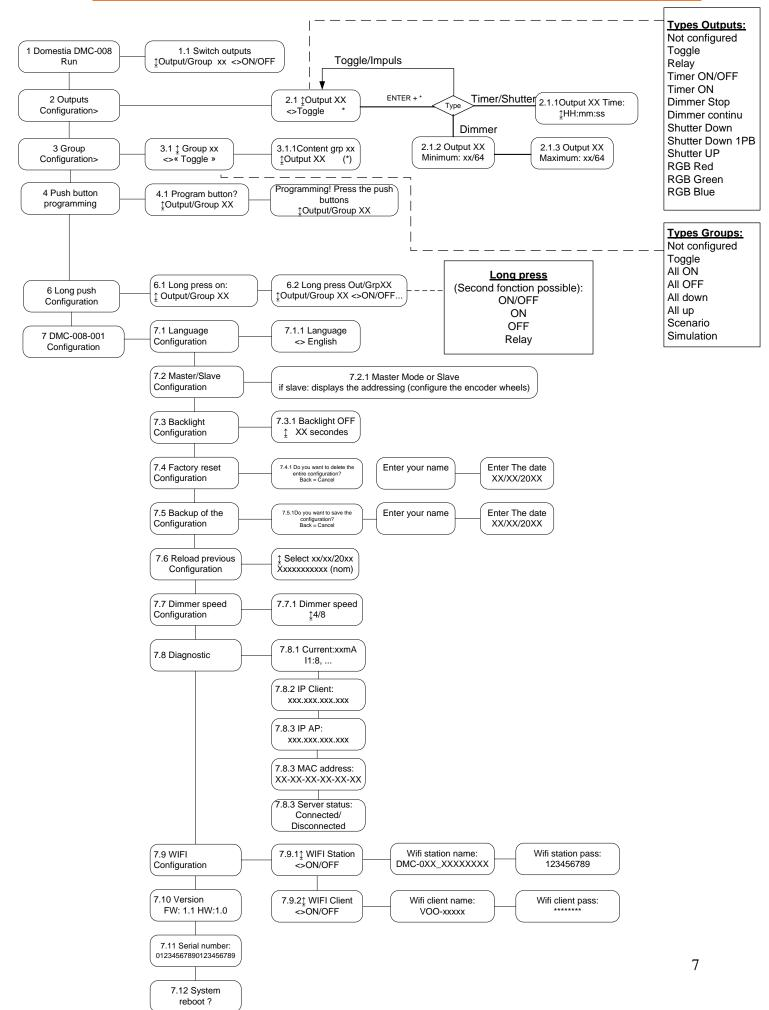
The DMC-012-003 is equipped with 6 buttons for programming with visualisation via a LCD screen. Navigation in the menus is as follows:
